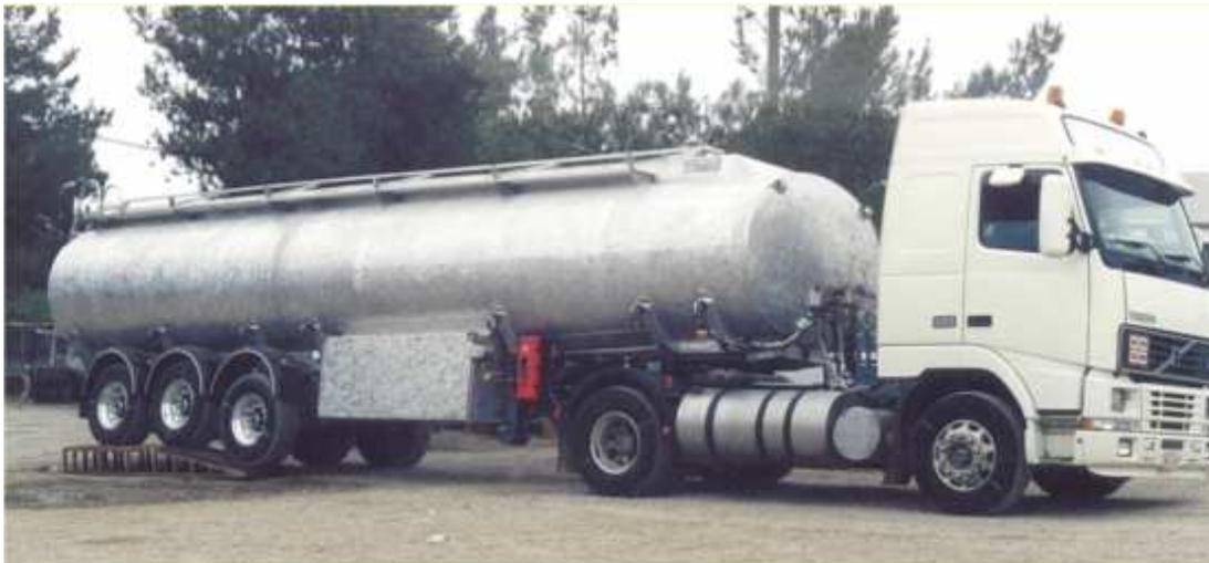
Torsional rigidity test for the first Made in Greece aluminum ADR tank (Jet Engineering SA)
