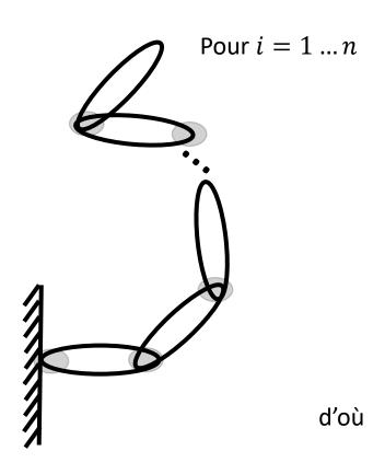
$$\frac{d}{dt} \frac{\partial T}{\partial \dot{q}_{i}} - \frac{\partial T}{\partial q_{i}} + \frac{\partial E_{p}}{\partial q_{i}} = Q'_{i}$$
