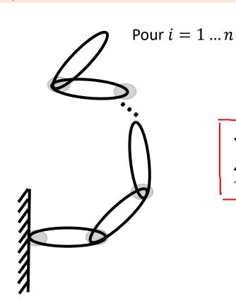
$$\frac{d}{dt}\frac{\partial T}{\partial \dot{q}_i} - \frac{\partial T}{\partial q_i} + \frac{\partial E_p}{\partial q_i} = Q_i'$$
